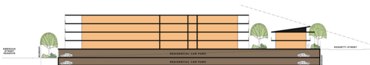
Figure 2: Scenario 1 Mixed use, shop top housing development: Progressive setback to Rossetti Street for mixed use development containing residential accommodation.
