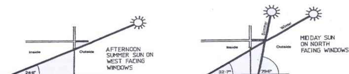
Sun Penetration through Windows Exclude hot afternoon summer sun by shading west & southwest facing windows
